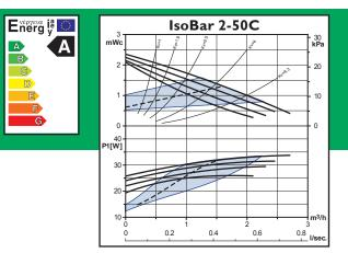
Classified in energy class A the IsoBar 2-50C, is the latest addition to our range of circulators and with capacities suitable for many properties. Up to 180m<sup>2</sup>, it is the ideal solution for many properties.
