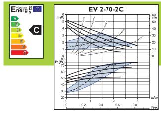
Domestic circulators are designed for efficiency and minimum energy consumption. The materials used are environmentally friendly. The rotor is encased in stainless steel, with a stainless steel shaft and carbon bearings, assuring quiet operation and long life.
