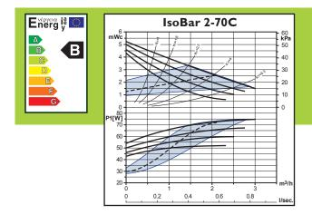
Isobar self-regulating circulators from Smedegaard are the answer to energy waste and velocity noise in heating installations. The IsoBar circulator is automatically self-adjusting in relation to the requirement of the installation. IsoBar circulators are designed with the Smedegaard I-2-3 motors, providing economic, environmental and technical advantages.
